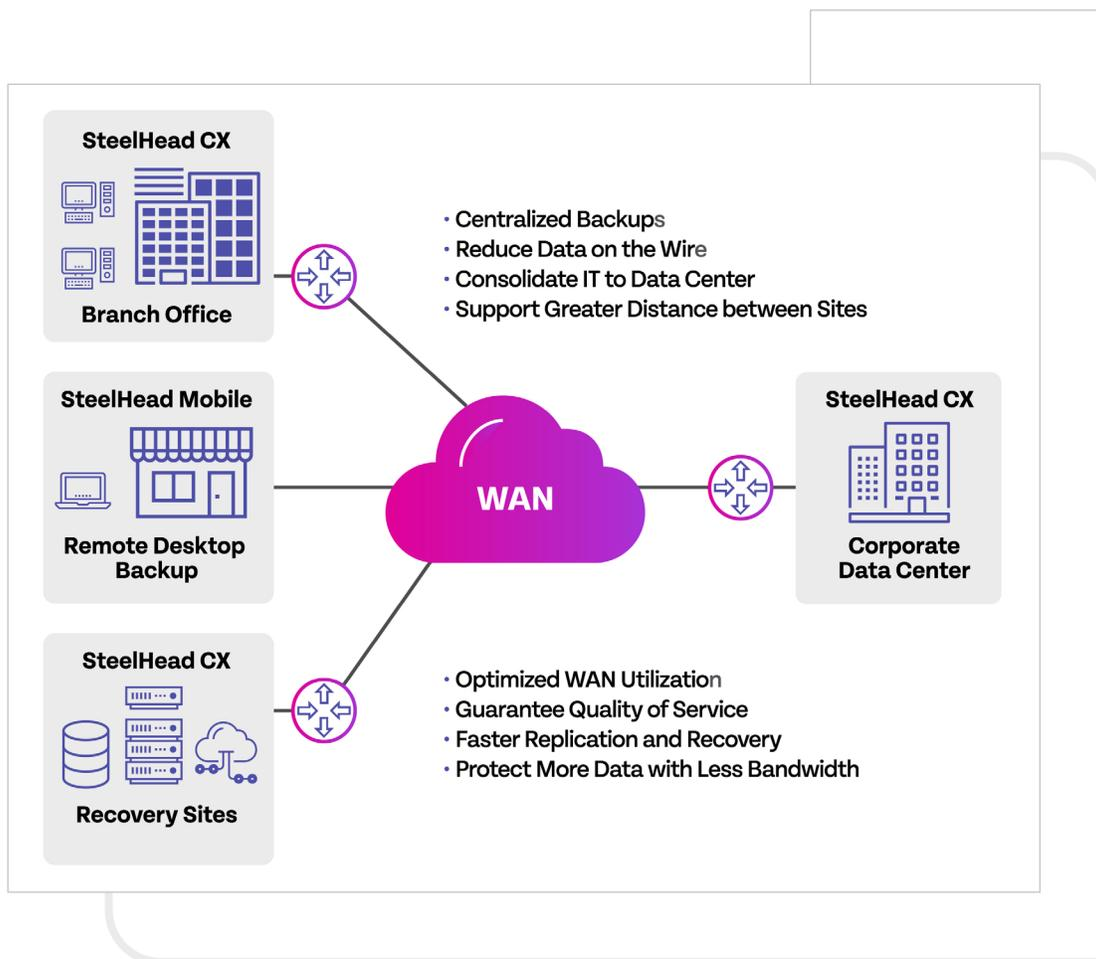
WAN-Optimized Disaster Recovery Reference Architecture (based on Riverbed® SteelHead™ family). Appliances are deployed at branch offices, remote desktops, disaster recovery sites, and in the primary data center, working transparently over the existing WAN to accelerate performance and maximize throughput.
