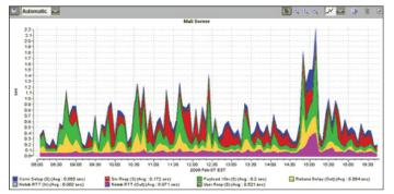
The AppResponse Response Time Composition Chart breaks down end-to-end application response into its component parts: TCP setup time, server response time, network time, time lost to packet loss, and latency, enabling network managers to very quickly distinguish between server, network, and application problems.
