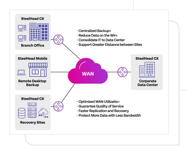
WAN-Optimized Disaster Recovery Reference Architecture (based on Riverbed® SteelHead™ family). Appliances are deployed at branch offices, remote desktops, disaster recovery sites, and in the primary data center, working transparently over the existing WAN to accelerate performance and maximize throughput.
