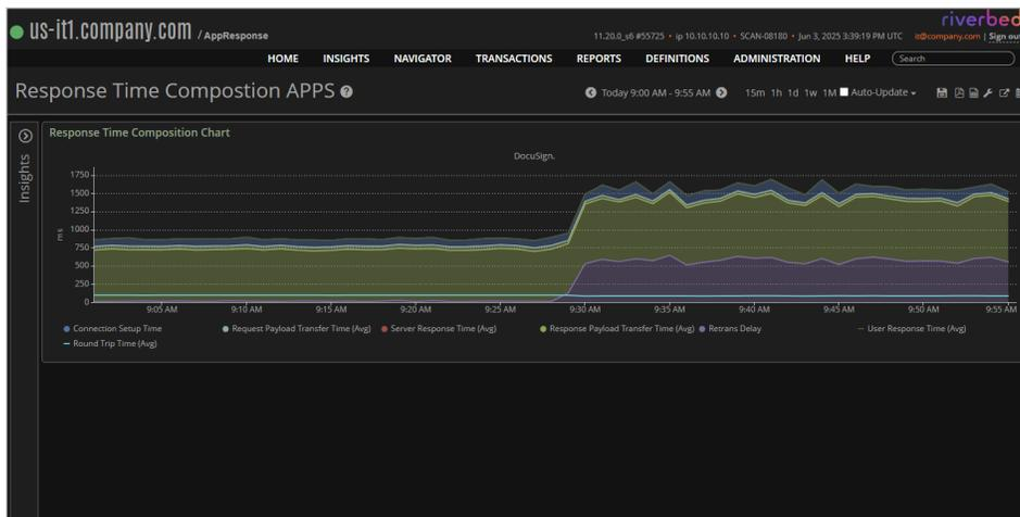
**Figure 1:** This AppResponse Response Time Composition Chart pinpoints delay sources across client, server, and network layers to accelerate root-cause analysis.
