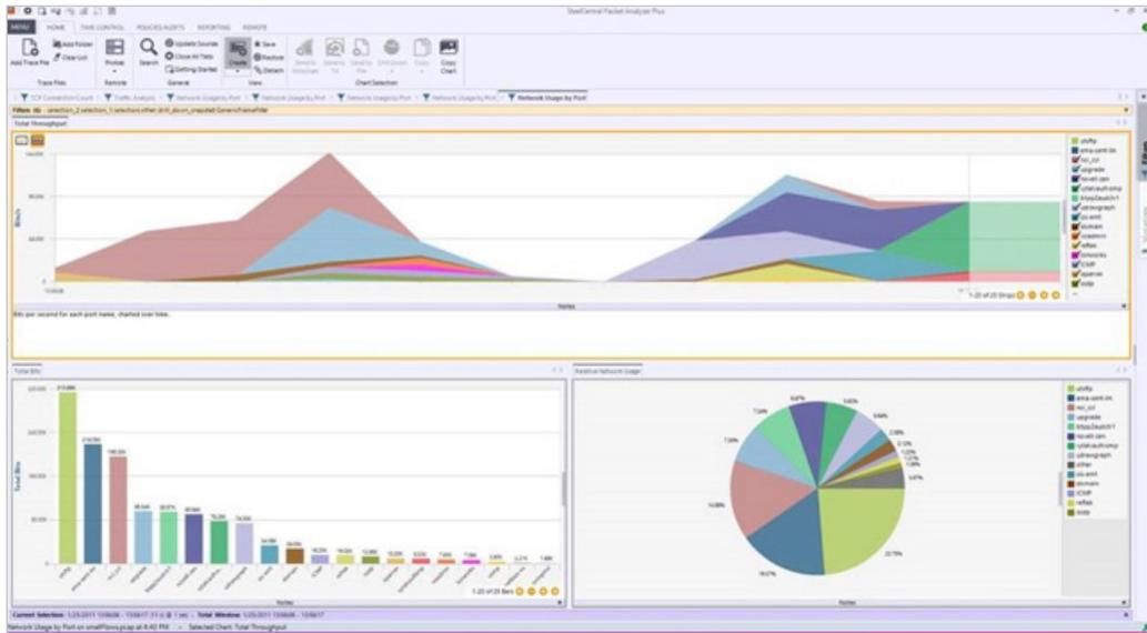
**Figure 1:** This is an example of a series of “views” that have been dropped on a local trace file or packets on a Riverbed AppResponse and the resulting analysis in Riverbed Packet Analyzer Plus. Because of the smart indexing that occurs at the time the packets are captured, the analysis happens almost instantaneously.
