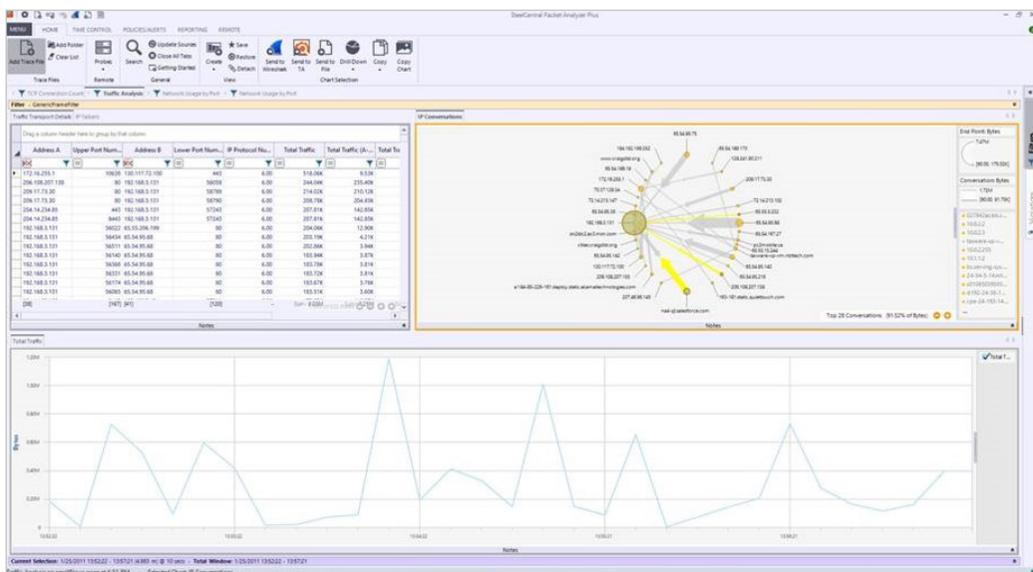
**Figure 2:** The conversation ring shows traffic between two nodes and displays it as a bidirectional stream; users can select either direction or both for analysis..
