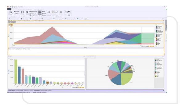
Figure 1: This is an example of a series of "views" that have been dropped on a local trace file or packets on a Riverbed AppResponse and the resulting analysis in Riverbed Packet Analyzer Plus. Because of the smart indexing that occurs at the time the packets are captured, the analysis happens almost instantaneously.
