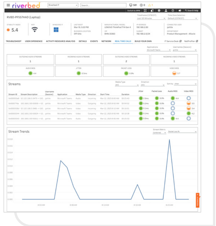
Figure 2: The UC Module offers real-time monitoring of voice and video performance metrics for all major collaboration platforms.
