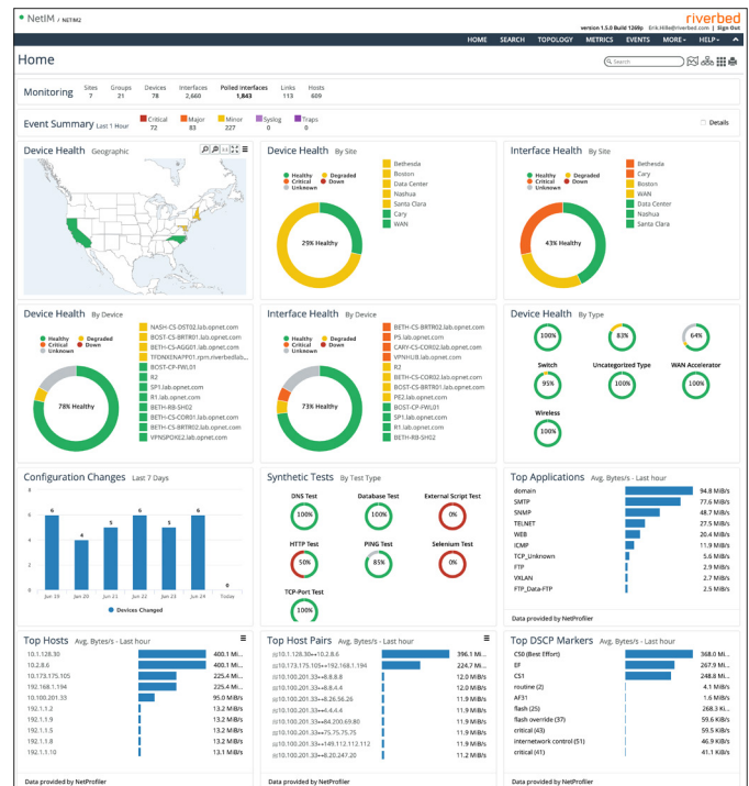
Figure 2: Home page enables you to visualize infrastructure performance by site, device, and by type.
