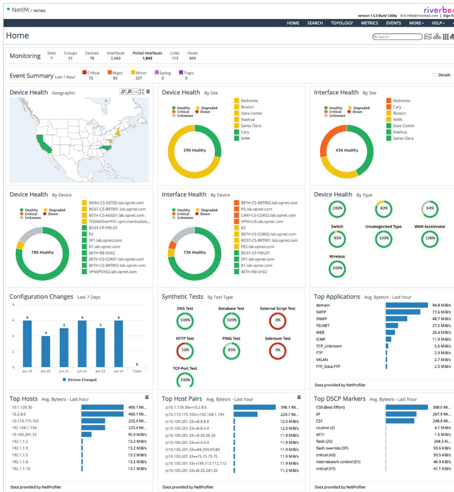
Figure 2: Home page enables you to visualize infrastructure performance by site, device, and by type.
